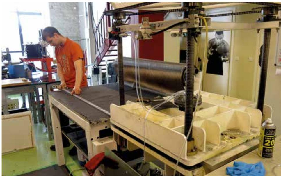
▲ Tamme invests heavily in R&D, not just for the products, but also for the manufacturing processes. In the foreground is a custom-built machine to ensure the best resin infusion
